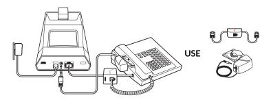
**IMPORTANT** *Cisco* phones use configuration **D** on the bottom of the base. Most other phones use default configuration **A**.
