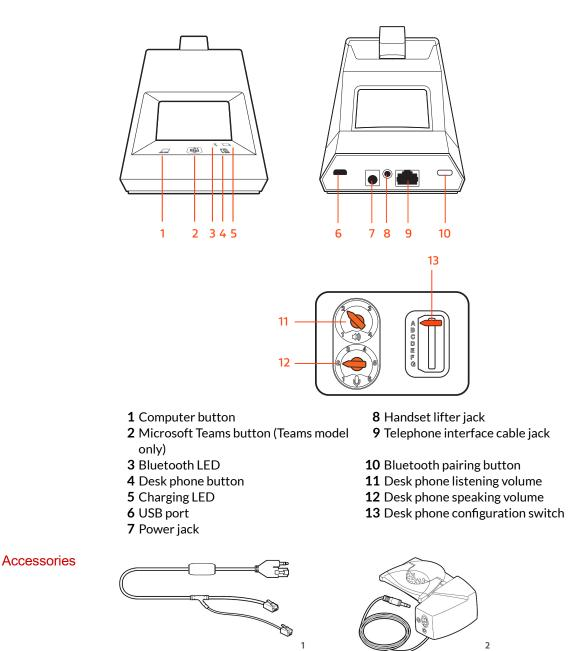
**1Electronic hookswitch cable (EHS cable)** Electronically and automatically answers/ends a desk phone call. Enables remote call control with your headset.
